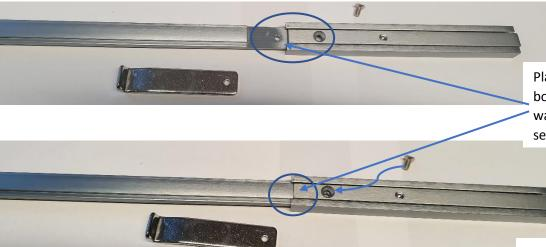
Place the end of the extension bolt into the slot where the tab was and screw the screw securely
